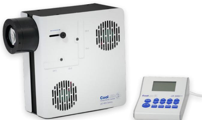
Individual control of four channels maximises image quality and can be operated via manual control pod, third-party imaging software or The LightBridge graphical user interface.
